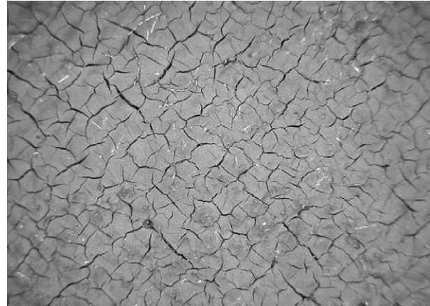
Fig. 2 – The surface morphology of the presented carbon cloth after MPL coating (using a digital microscope with the magnification, 50×).
